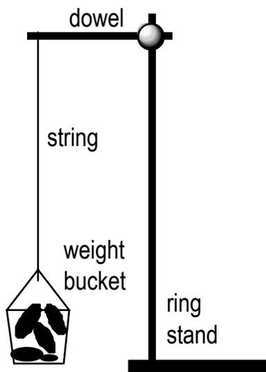
apparatus consists of a ring stand, a wooden dowel attached to the ring stand by means of a clamp, a string with one end attached to the end of the dowel and the other end attached to a small bucket, and gravel to be used to add weight to the bucket. The instructor will discuss the basic use of the pendulum, including how to change some of the variables, such as weight and length.
